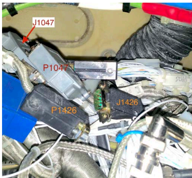
Figure 1. Connector locations for Avidyne equipped Cirrus
